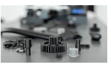
Powder metallurgically produced components play an important role in industry. Their advantages lie in their high dimensional accuracy and their wide range of densities, from highly porous to highly dense. The density of the workpieces plays a decisive role here. For example, the bulk density of the powder influences the strength, porosity and other parameters of the moulded part. The aim is to eliminate blowholes or similar defects that affect the porosity and stability of the components.
