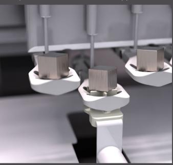
analyse co-printed density cubes. These can be analysed quickly and precisely. The density obtained is compared with the stored characteristic data and, thanks to direct correlation, the porosity of the component can be calculated.
